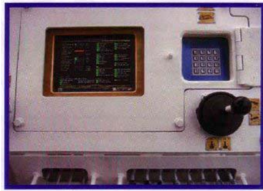
PLC display and keypad
